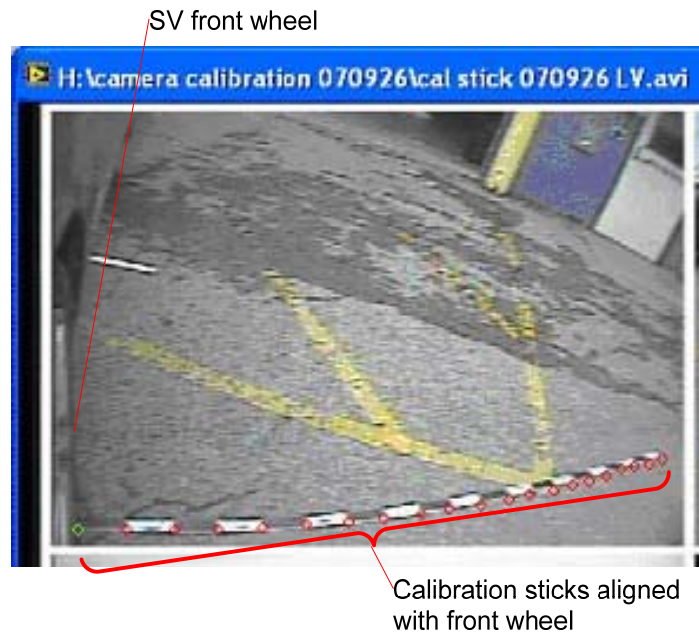
Figure 6. Calibration of side camera using meter sticks.
