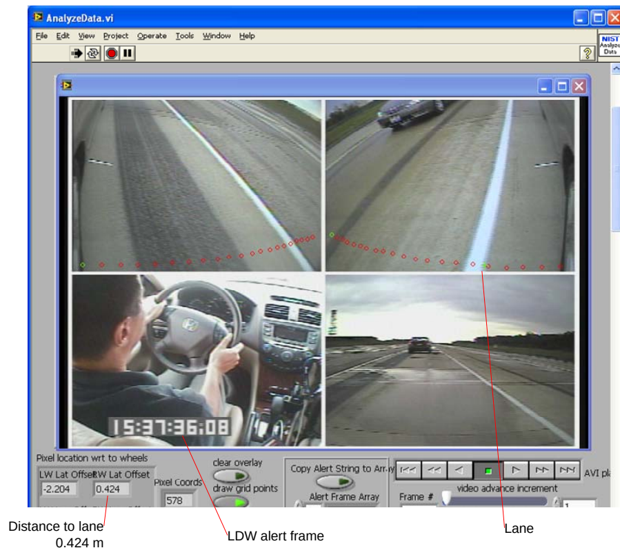
Figure 11. Measuring lateral distance to lane at time of warning.
