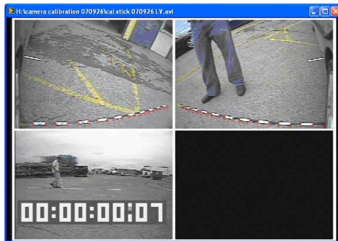
Figure 25. Calibration sticks with 10 cm marks adjacent to left and right front wheel.
